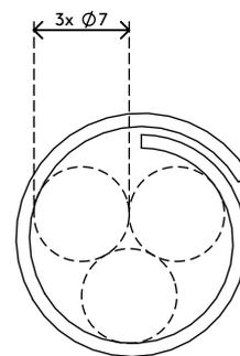
Addit bobina mangiacavo  $\varnothing 15$  mm/25 m 712
