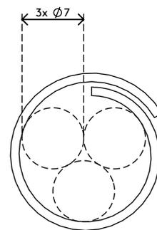
Addit Kabelschlucker Ø15 mm/25 m 713
