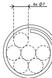
Addit Kabelschlucker  $\varnothing 25$  mm/20 m 761
